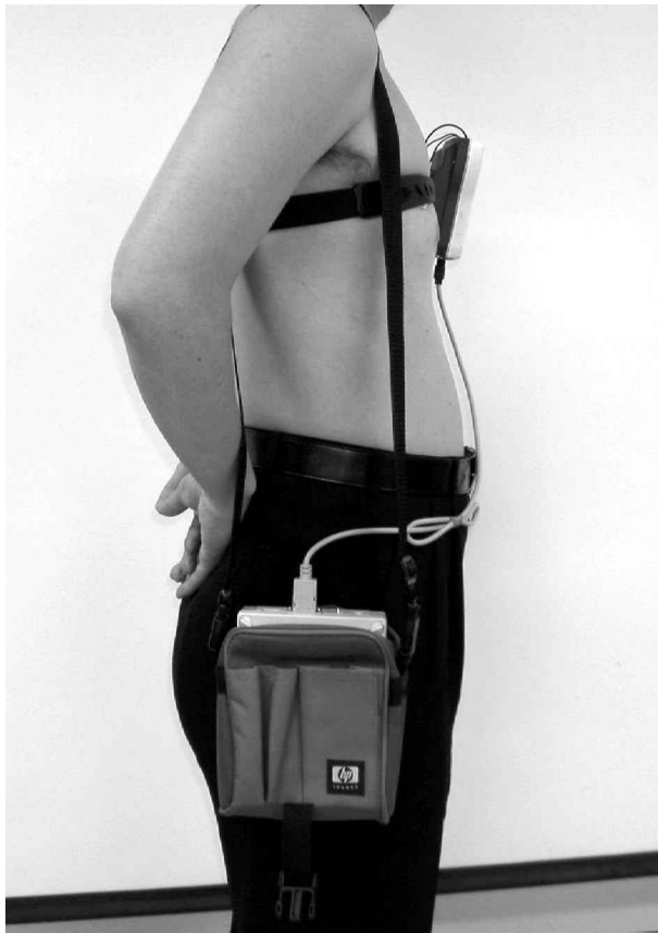
Fig 5 A person wearing the Bluetooth-based communication system. Because of the embedded LINUX board, the system is rather bulky (compare Fig 1).
