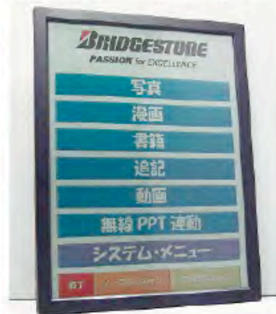
Fig 4 E Ink Goes Color A number of particle-based type color ePaper designs are expected to go commercial in 2009 and 2010. (a) The color ePaper from E Ink, with an enlarged view (b). The RGBW color filters are visible. Bridgestone is also implementing color display using RGBW color filters (c).
