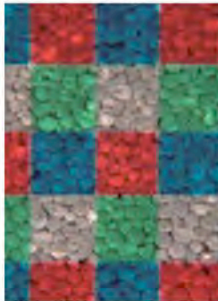
Fig 4 E Ink Goes Color A number of particle-based type color ePaper designs are expected to go commercial in 2009 and 2010. (a) The color ePaper from E Ink, with an enlarged view (b). The RGBW color filters are visible. Bridgestone is also implementing color display using RGBW color filters (c).
