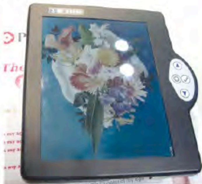
Fig 4 E Ink Goes Color A number of particle-based type color ePaper designs are expected to go commercial in 2009 and 2010. (a) The color ePaper from E Ink, with an enlarged view (b). The RGBW color filters are visible. Bridgestone is also implementing color display using RGBW color filters (c).
