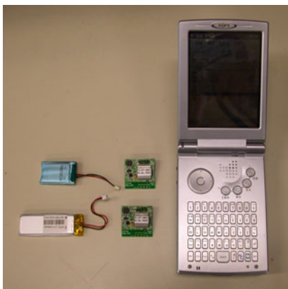
Fig. 4. The picture of the platform showing two scm with varying battery and the central monitoring unit.
