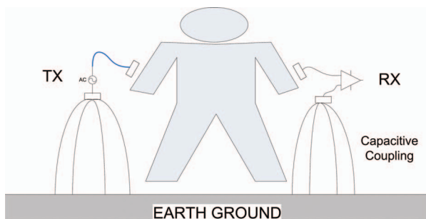
Figure 1. Near-field intra-body communication proposed by Zimmerman
