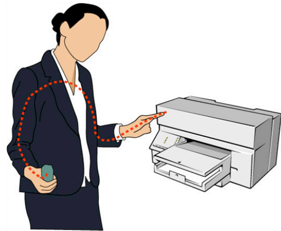
Figure 1. Using TAP, which enables the user to print the desired photo in the camera by touching the printer while holding the digital camera
